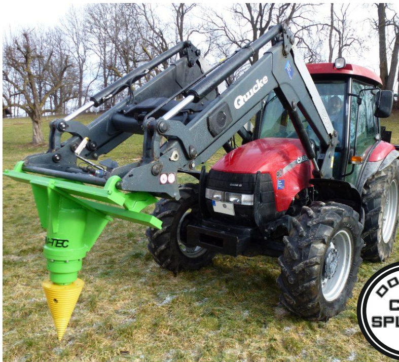
cone wood splitter - with attachment for front- or wheel loaders
