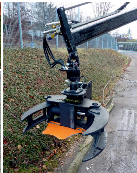
energy wood grapple with hydr./fixed knife / with tilt function or rigid attachment
