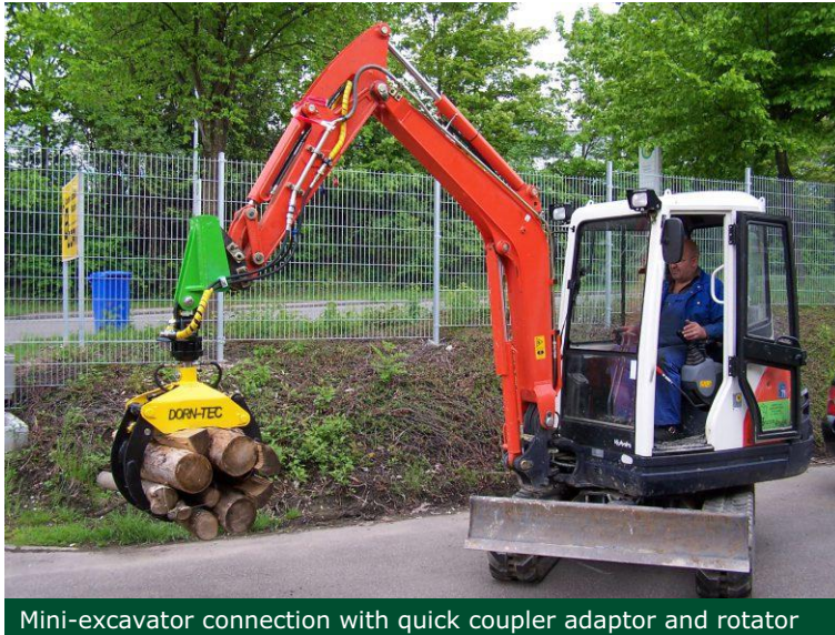
Mini-excavator connection with quick coupler adaptor and rotator
