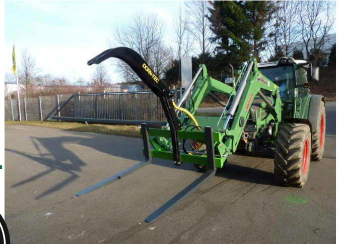
hydr. downholder with big opening for firewood bundles
