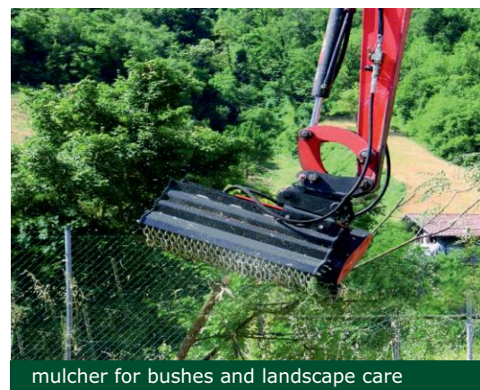
hydraulic mulcher with mechanical side shift
