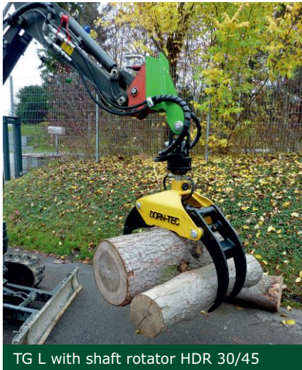
Mini-excavator connection with quick coupler adaptor and rotator
