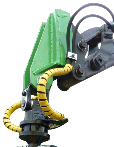
Q-coupler adapter with linkage
