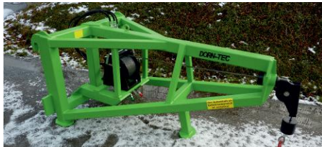
mounted winch with extension frame
