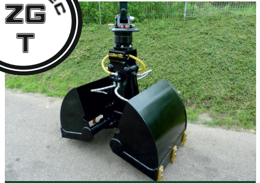
strong clamshell bucket for digging operations
