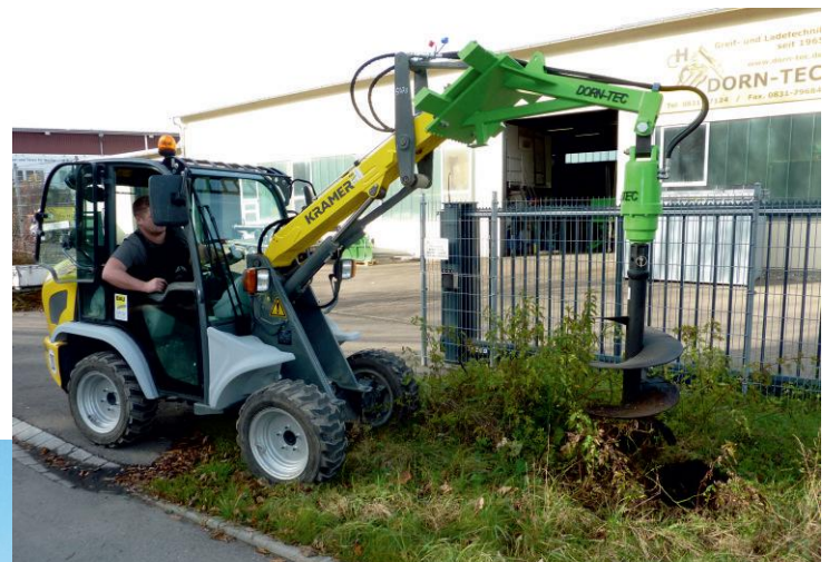
auger with adapter for a wheel loader made by DORN-TEC
