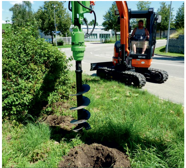
classic excavator application with quick-change adapter
