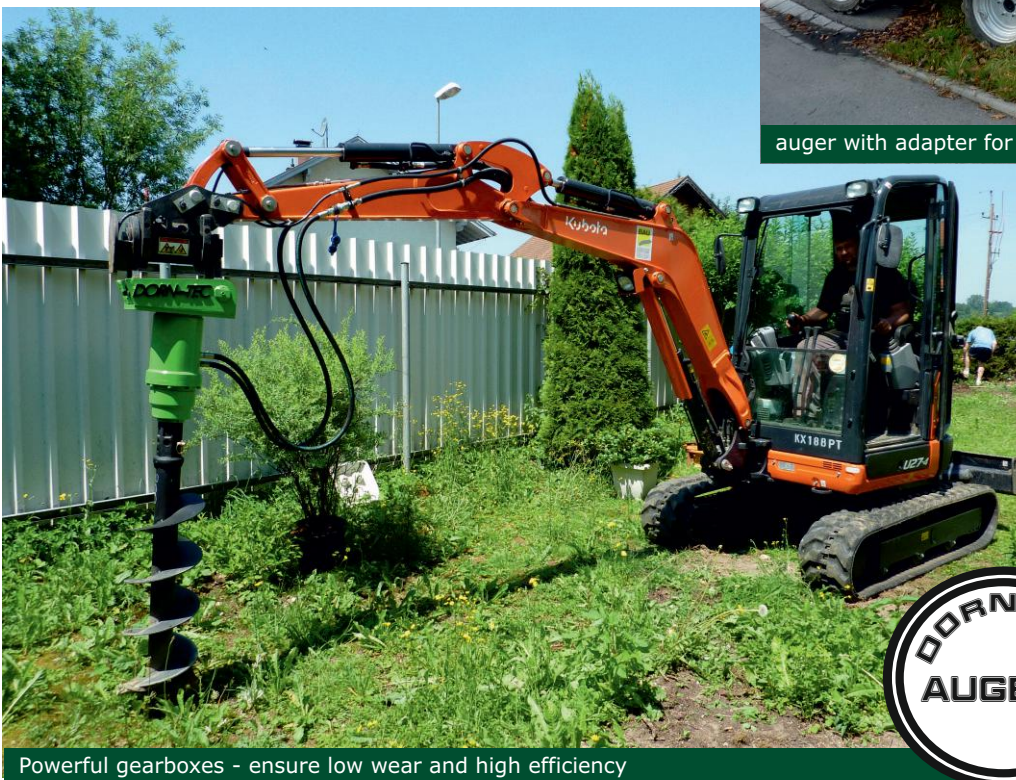
auger with fork shoe adapter / solid auger worms
